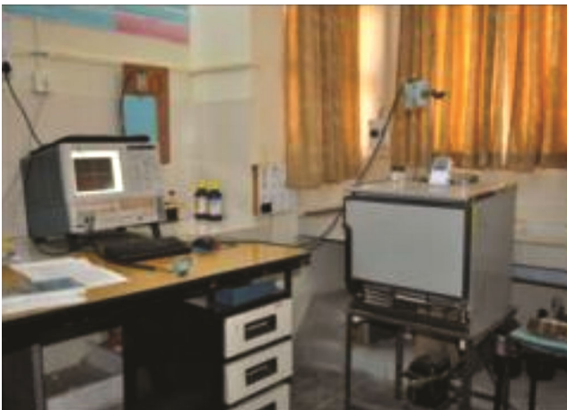
Fig. 2 — Experimental set up of time domain dielectric technique (TDDT).
