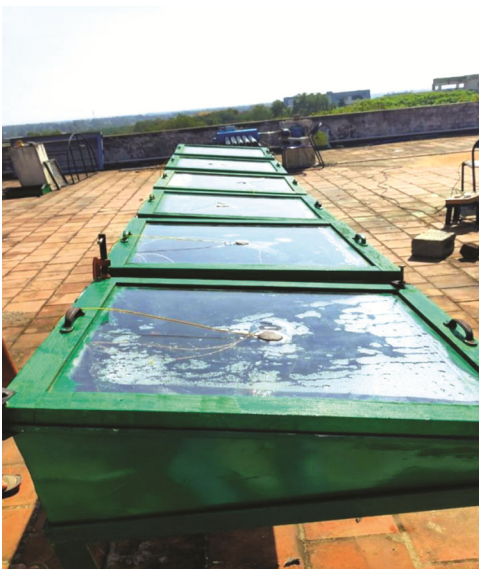
Fig. 1 — Experimental setup of single slope solar still.
