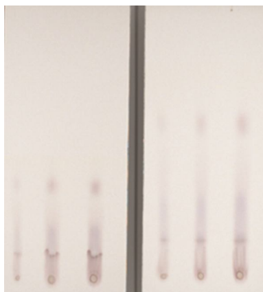
Fig. 7 — Qualitative TLC analysis (under white light) of anthocyanin enriched fraction
