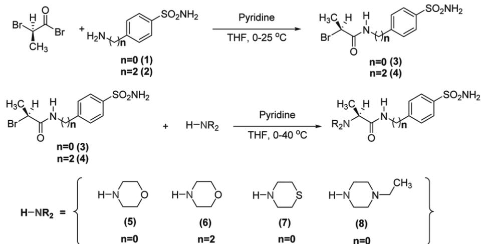
Scheme I — Reaction diagram for the synthesis of  $N^4$ -substituted aminobenzenesulfonamides **5-8**
