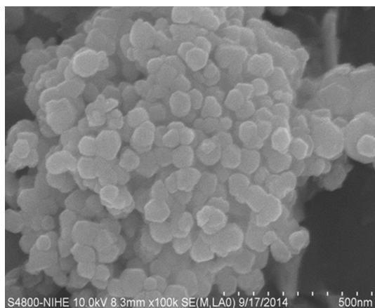
Figure 2 — SEM image of uncoated \text{Co}_{0.5}\text{Ni}_{0.5}\text{Fe}_2\text{O}_4
