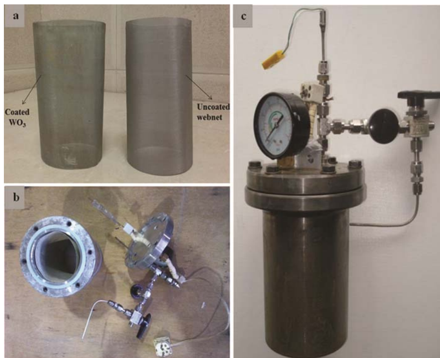
Fig. 1 — The present of (a) coated and uncoated cylindrical stainless steel webnets with \text{WO}_3 particles (b) open photocatalytic reactor with its cap and lamp situation and (c) the assemble photoreactor.
