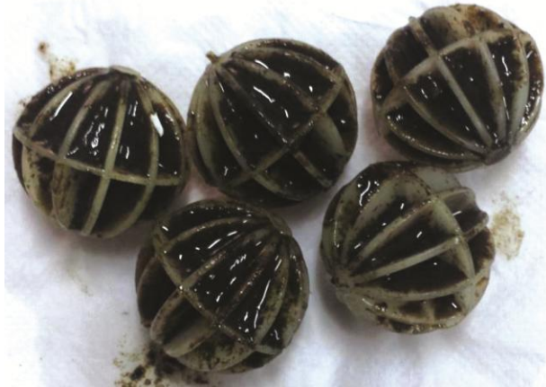
Fig. 3 — Photograph of the biomass accumulation on polypropylene spherical inert media.
