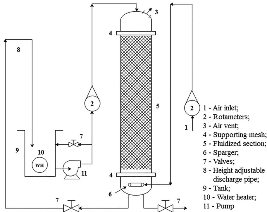
Fig. 1 — Schematic diagram of the IFBBR.
