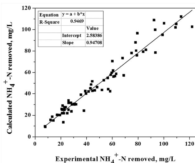
Fig. 5 — Comparison between calculated and experimental values for the amount of  $\text{NH}_4^+\text{-N}$  removed.
