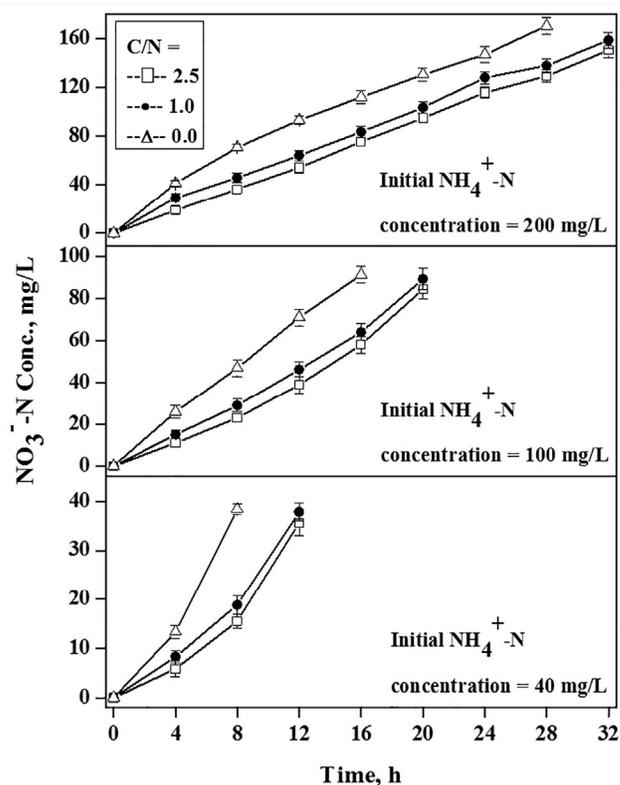
Fig. 3 — Effect of C/N ratios on the formation of  $\text{NO}_3^-\text{-N}$  for different initial  $\text{NH}_4^+\text{-N}$  concentrations.
