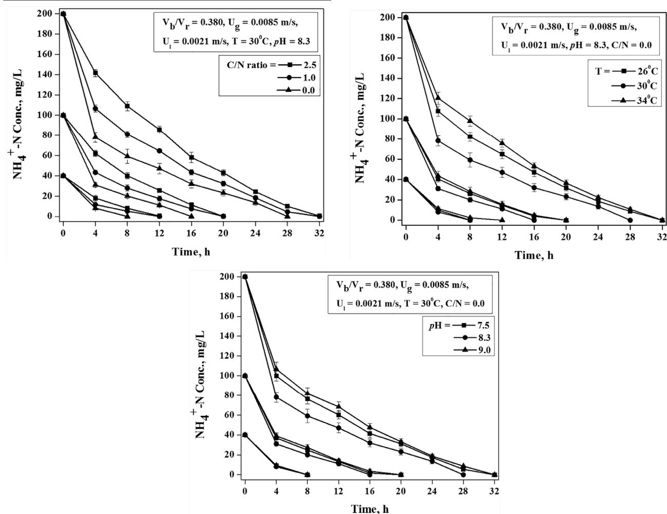
Fig. 2 — (a) Effect of C/N ratios, (b) temperature and (c) pH on the removal of  $\text{NH}_4^+-\text{N}$  for different initial  $\text{NH}_4^+-\text{N}$  concentrations.
