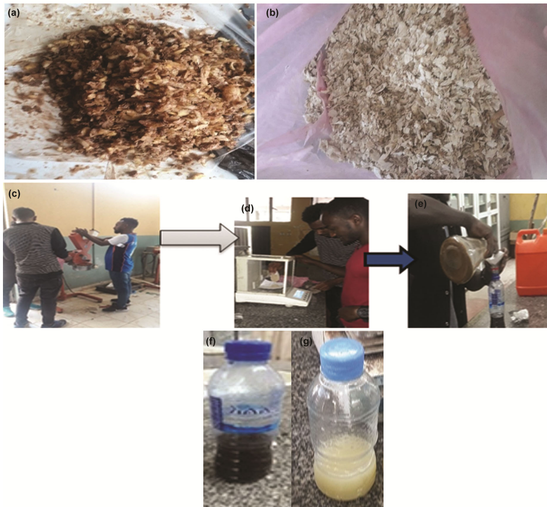
Fig. 1 — (a) Ginger peel (b) Garlic peel, (c-e) extraction process of the antimicrobial material, milling, solvent weighing and dissolving and filtration respectively from right to left, (f) final antimicrobial ginger peel extract and (g) garlic peel extract
