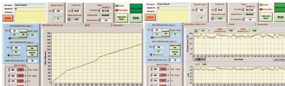
Fig. 4 — Wear parameters display on pin-on-disk rotary tribometer
