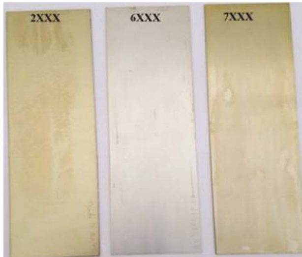
Fig. 4 — Photographic images of the anodized and sealed aluminium alloy specimens after 336 h of salt fog exposure.
