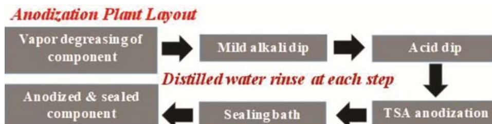
Fig. 1 — Chromic acid-free permanganate sealed TSA process layout.
