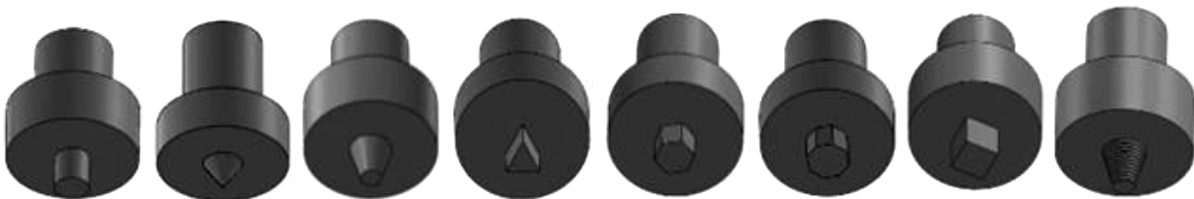
Fig. 4 — Different shapes of probe profile used in FSP.
