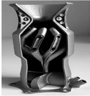
Fig. 11 — Consolidated assemblies as a single part 96 .
