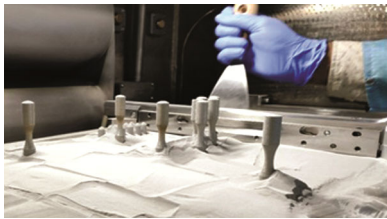
Fig. 12 — Removing the surrounding powder of finished part to use it for next product.
