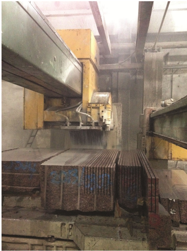
Fig. 1 — An overall view of the blocks cut and the block cutter from which power consumption values were obtained.
