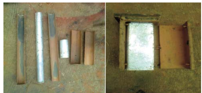
Fig. 1 — Clay coated actual mold used with cast MMCs.
