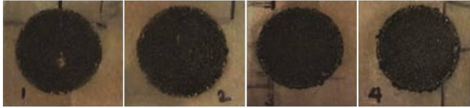
Fig. 2 — TiC-Cu coating deposited on AISI 304 stainless steel substrate by EDC process.
