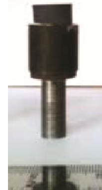
Fig.1 — TiC-Cu tool electrode prepared by P/M method after joining with mild steel tool extension.
