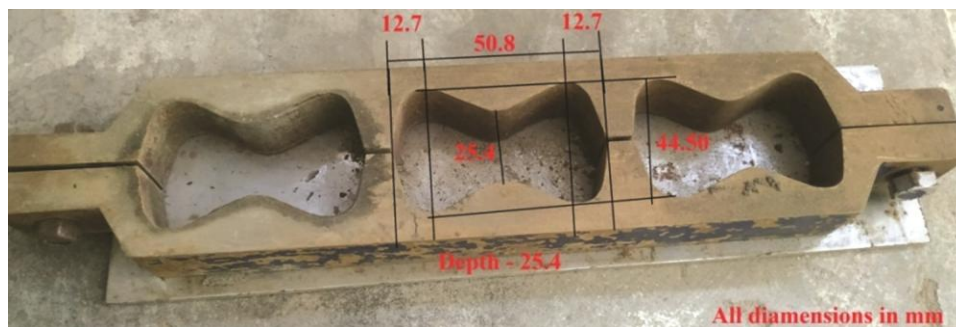
Fig. 7 — Briquette mould for specimens of split tensile strength test.
