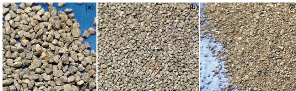
Fig. 2 — Different grades of recycled concrete fine aggregate (a) RCFA-I, (b) RCFA -II and (c) RCFA -III.
