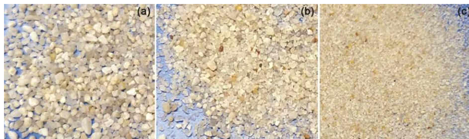
Fig. 1 — Different grades of natural standard sand (a) NSS-I, (b) NSS-II and (c) NSS-III.
