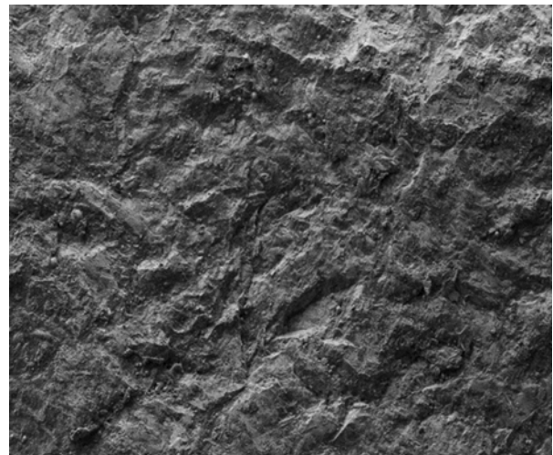
Fig.11 — SEM image of fracture surface in fatigue.
