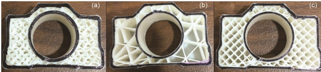
Fig. 7 — Infill patterns used in investigation; (Zigzag), (b) Triangles, and (c) Gyroid.
