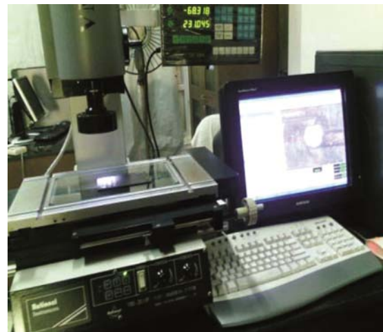
Fig. 4 — Setup of video measurement system.
