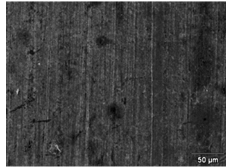
Fig. 13 — SEM micrograph of type 1 steel plasma coated under condition 2 (78% Ar).
