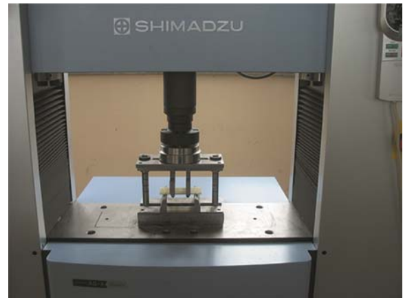
Fig. 3 — Flexural test with four-point bending fixture.
