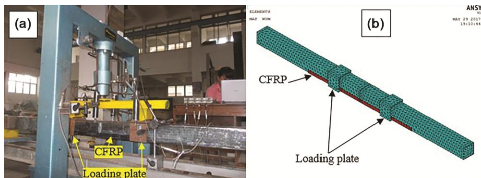
Fig. 2 — Comparison of beam C strengthened by CFRP sheet (a) Experimental 30 and (b) Numerical simulation
