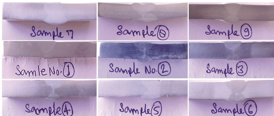
Fig. 5 — Macroscopic images of weld cross section.
