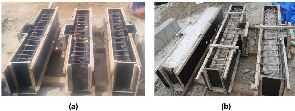
Fig. 5 — Process of preparing test beams (a) embedment of steel reinforcement cage in template, and (b) pouring of the first batch of concrete.
