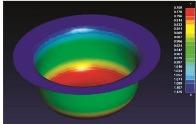
Fig. 10 — Thickness distribution in the sample after analysis.
