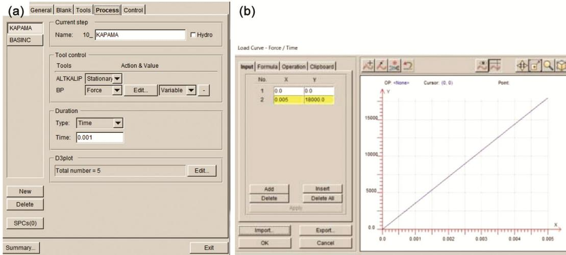
Fig. 5— a) Defining the closing process, and b) Defining the time-BHF curve.
