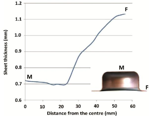
Fig. 11 — Thickness distribution of sheet metal obtained from FEA.
