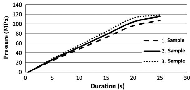
Fig. 12 — Change of pressure as a function of time for sheet thickness 1.0 mm (Experimental results).
