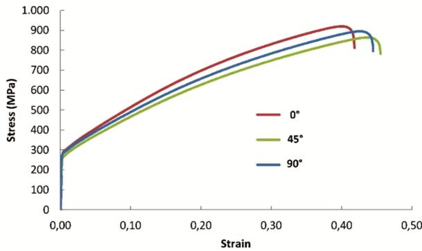
Fig. 8 — Change of true stress-strain curves according to rolling direction.
