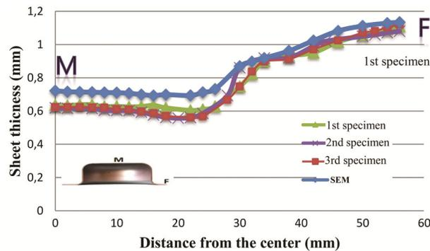
Fig. 13 — Comparison of thickness distributions obtained from experimental and FEA (for sheet thickness 1.0 mm).
