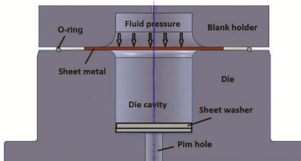
Fig. 1 — The die used on performing sheet hydroforming process with female die.
