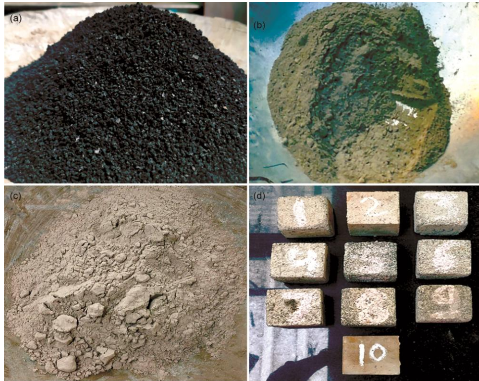
Fig. 1 — Materials used in development of the composite matrix a) Tyre rubber granules, b) Cement, c) Fly ash, and d) Composite matrix with varied combination of a , b and c.
