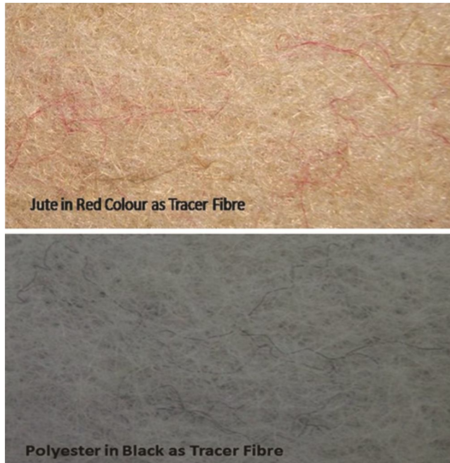
Fig. 2 — Arrangement of tracer fibres in 100% jute and 100% polyester nonwoven fabrics
