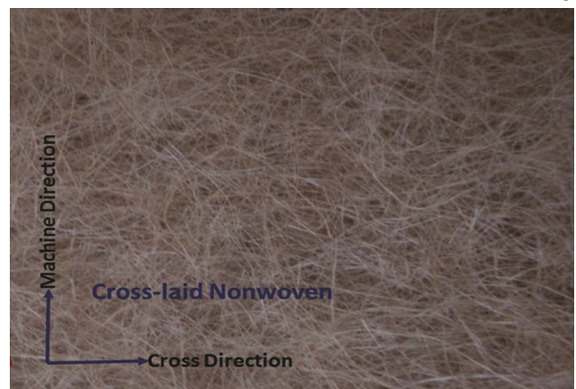
Fig. 7 — Orientation of fibres in jute-polyester cross laid needle punched fabric
