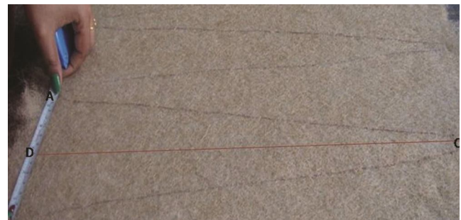
Fig. 4 — Measurement of actual laying angle using straight filament yarn
