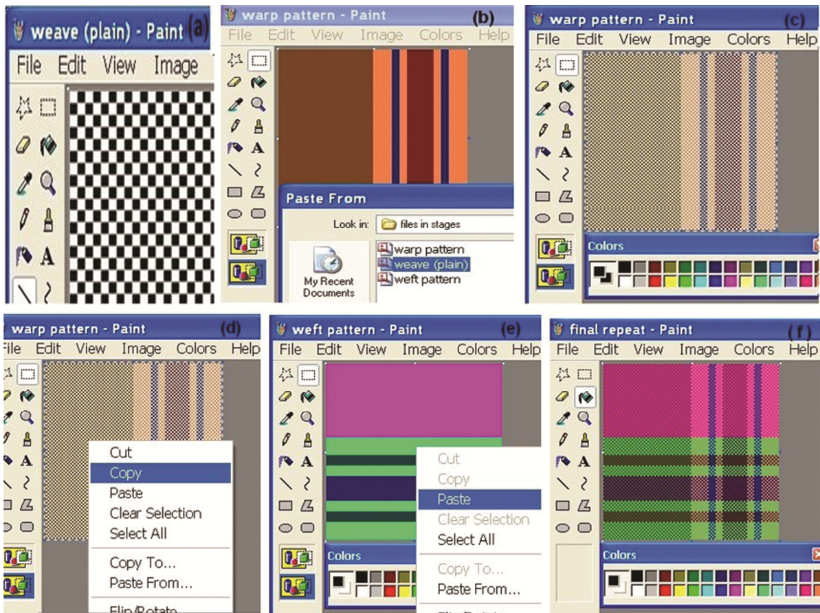
Fig. 4 — Different steps in merging the weave file with colour pattern file
