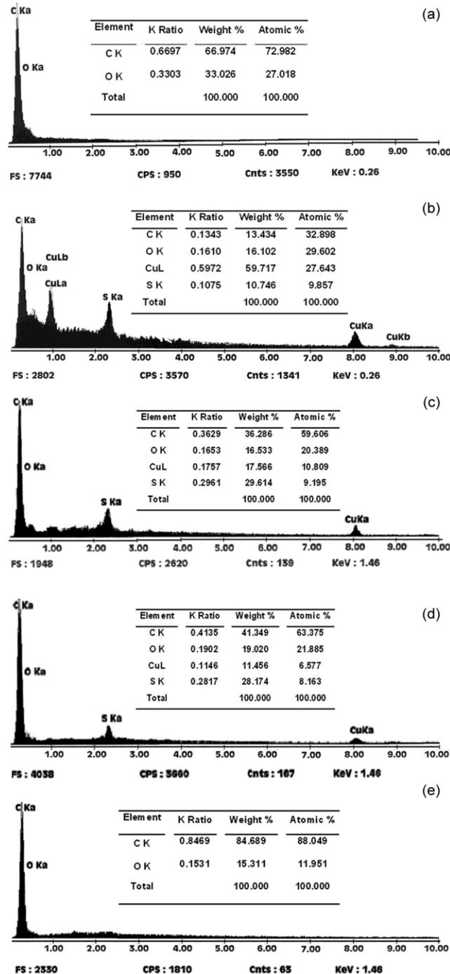
Fig. 4 — An elemental analysis on the cross-section of the coated acrylic fibres by 2  $\mu\text{m}$  intervals: (a) uncoated samples, (b) surface of coated samples, and the depth of 2 (c), 4 (d), and 6 (e)  $\mu\text{m}$  from the surface of the coated samples
