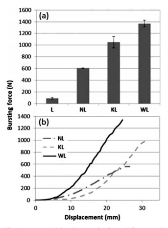
Fig. 4 — Average (a) bursting strength values and (b) curves of bursting load – displacement
