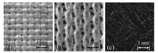
Fig. 1 — Magnified images of the reinforcing fabrics' surfaces (a) woven, (b) knitted, and (c) nonwoven
