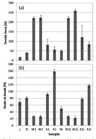
Fig. 2 — (a) Average values of tensile load and (b) strain at break for raw materials and synthetic leather samples
