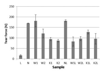
Fig. 3 — Average values of tear load for raw materials and synthetic leather samples
