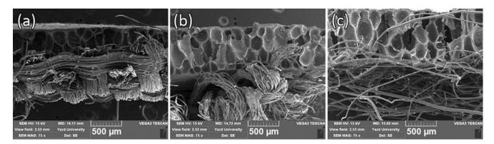
Fig. 5 — SEM images of fractured surfaces of the samples (a) WL, (b) KL and (c) NL
