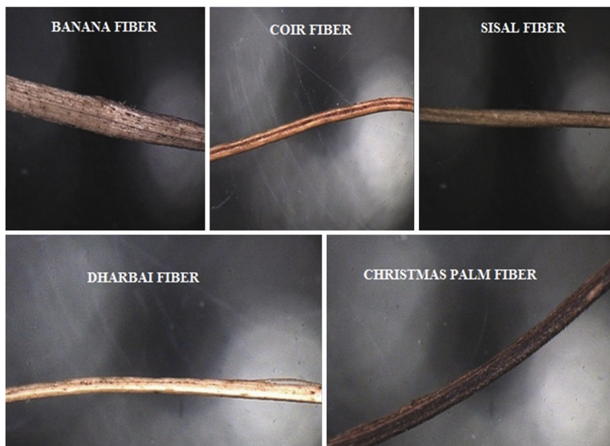
Fig. 1—Diameter measurement of natural fibres
