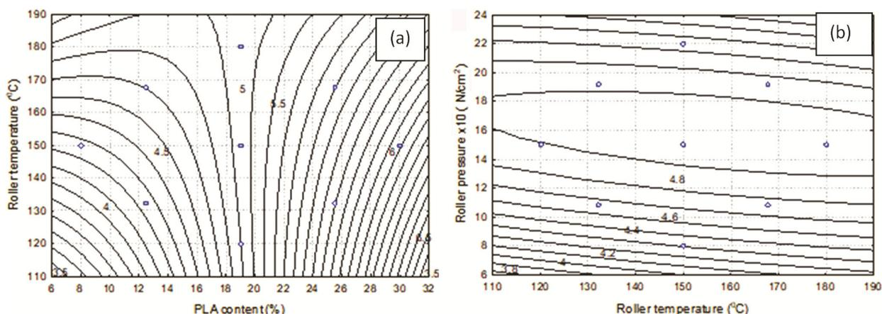
Fig. 7 — Tear strength of jute-PLA fabric (a) effect of PLA% and temperature for 150 N/cm<sup>2</sup>; and (b) effect of temperature and pressure for 19% PLA content
