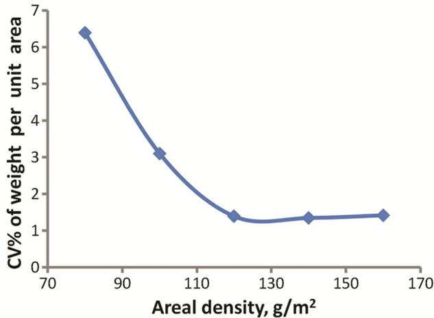
Fig. 8 — Irregularity of thermo-bonded fabric
