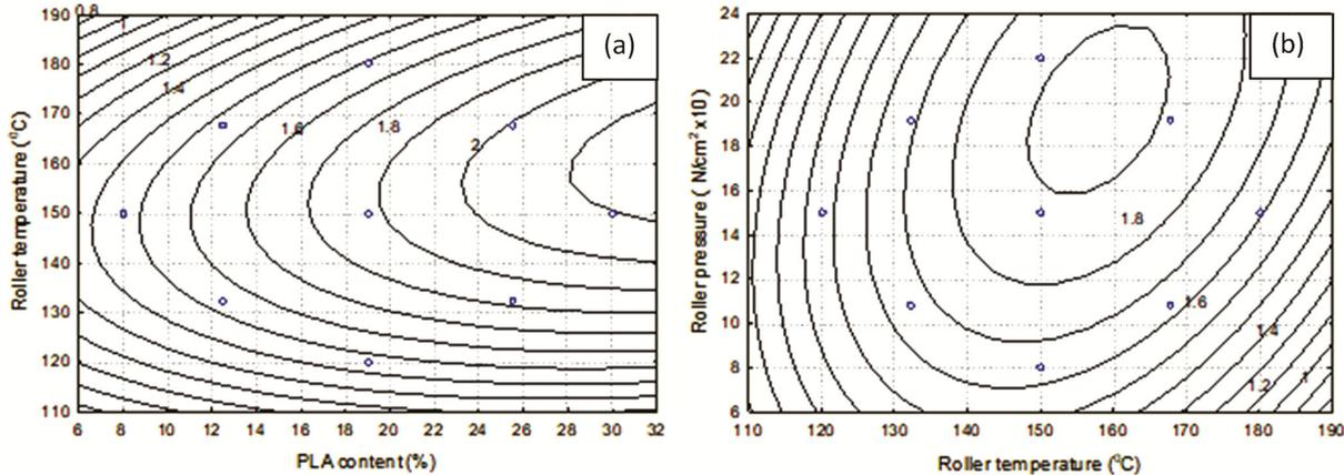
Fig. 3 — Tenacity of jute-PLA fabric, (a) effect of PLA% and temperature for 150 N/cm<sup>2</sup> pressure, and (b) effect of temperature and pressure for 19% PLA content
