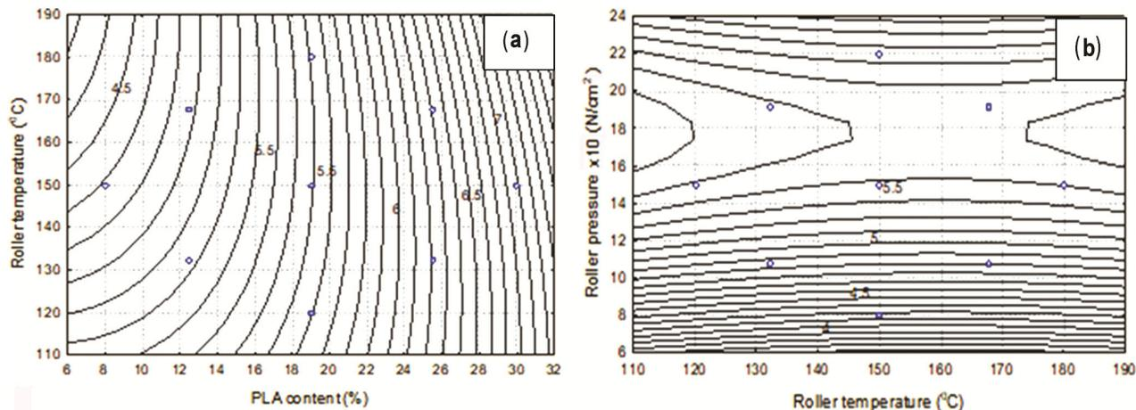
Fig. 6 — Bursting strength of jute-PLA fabric (a) effect of PLA% and temperature for 150 N/cm<sup>2</sup>; and (b) effect of temperature and pressure for 19% PLA content
