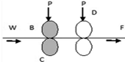
Fig. 1 — Schematic diagram of thermal bonding machine (W – fibre web, P – pneumatic pressure, B – hot roller with dot surface, C – hot roller with smooth surface, D – cold roller with smooth surface, and F- bonded fabric)
