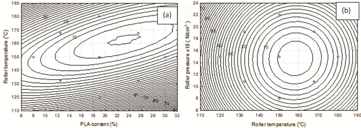
Fig. 4 — Extension-at-break of jute-PLA fabric (a) effect of PLA% and temperature for 150 N/cm<sup>2</sup>; and (b) effect of temperature and pressure for 19% PLA content
