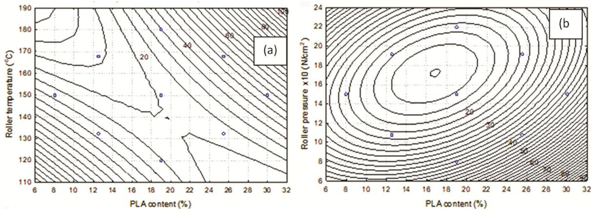
Fig. 5 — Initial modulus of jute-PLA fabric (a) effect of PLA% and temperature for 150 N/cm<sup>2</sup>; and (b) effect of PLA% and pressure for 19% PLA content
