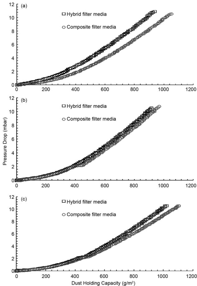
Fig. 6 — Evolution of pressure drop with dynamic loading of dust in case of composite and hybrid filter media, (a) equal proportion of round and trilobal fibres, (b) equal proportion of round and deep-grooved fibres and (c) equal proportion of round, trilobal and deep-grooved fibres
