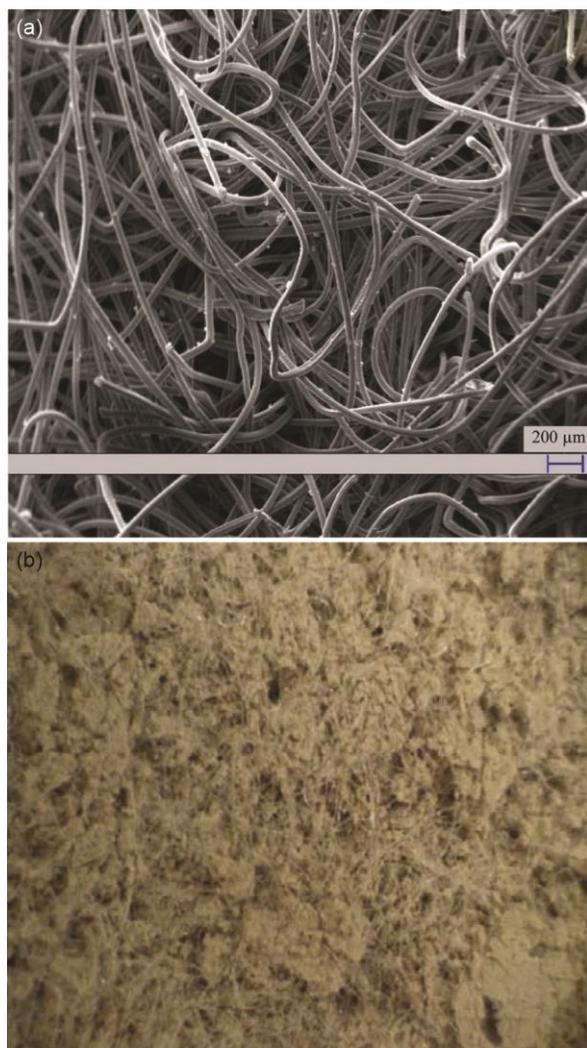
Fig. 4 — Composite filter media prepared from 19.13  $\mu\text{m}$  and 30.17  $\mu\text{m}$  polypropylene fibres, (a) before dust loading and (b) after dust loading
