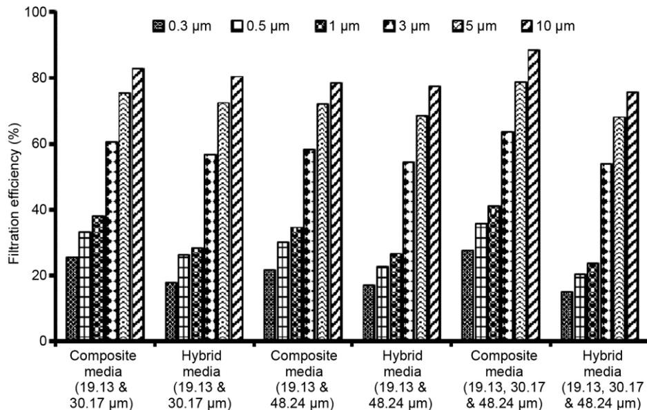
Fig. 2 — Comparison of filtration efficiency of composite filter media and hybrid filter media made up of fibres of different sizes
