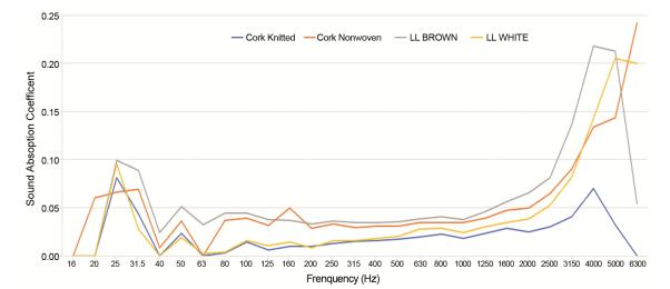
Fig. 5 — Sound absorption properties
