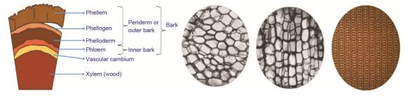
Fig. 1 - Cross-section of cork bark and laminated knitted backing layer
