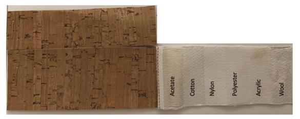
Fig. 4 — Color fastness test result of knitted backed cork leather
