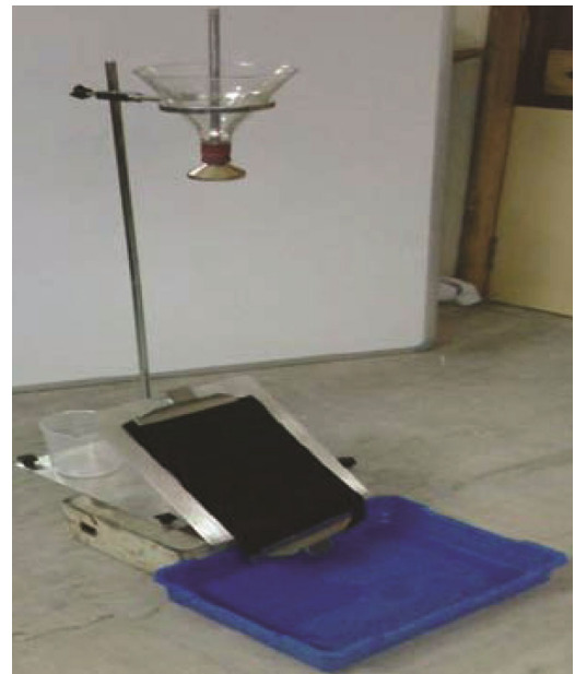
Fig. 6 — Spray impact penetration test
