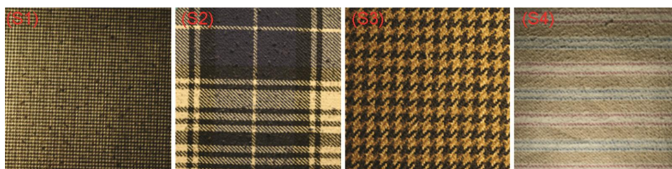
Fig. 1—Images of patterned samples after pilling resistance test
