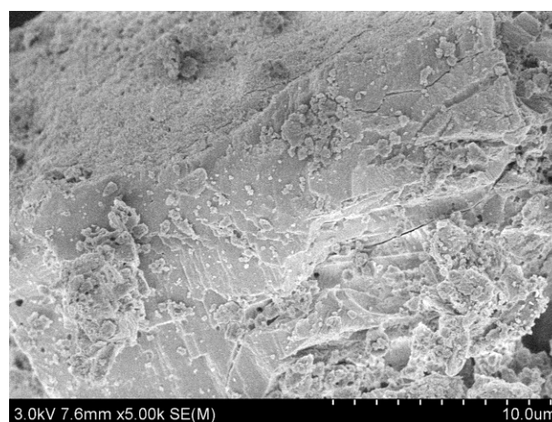
Fig. 3 — SEM image of uncalcined egg shells
