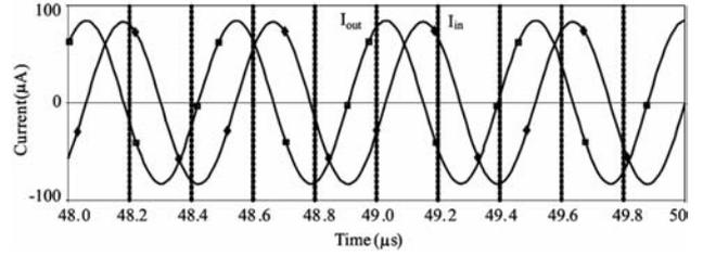
Fig. 9 — Time-domain response of the APF at a 2.06 MHz sinusoidal input signal
