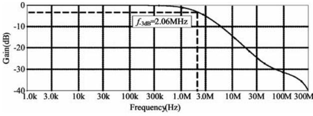
Fig. 5 — Frequency response of the CMOS OA
