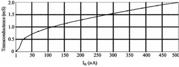
Fig. 6 — Transconductance value of the CMOS OTA relative to  $I_B$
