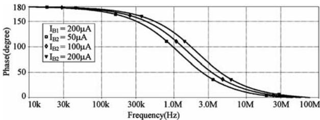
Fig. 8 — Phase response of the APF for different value of  $I_{B2}$
