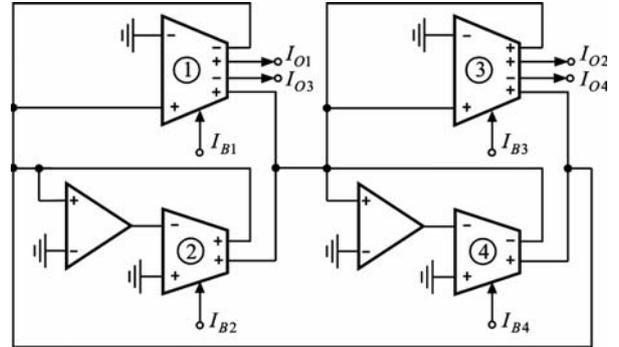
Fig. 3 — Proposed current-mode quadrature oscillator
