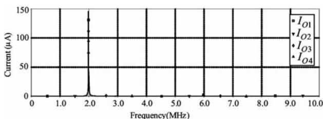
Fig. 14 — Output spectrum of quadrature oscillator
