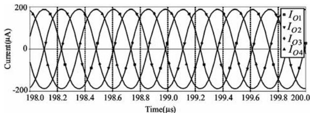
Fig. 13 — Output waveforms of quadrature oscillator
