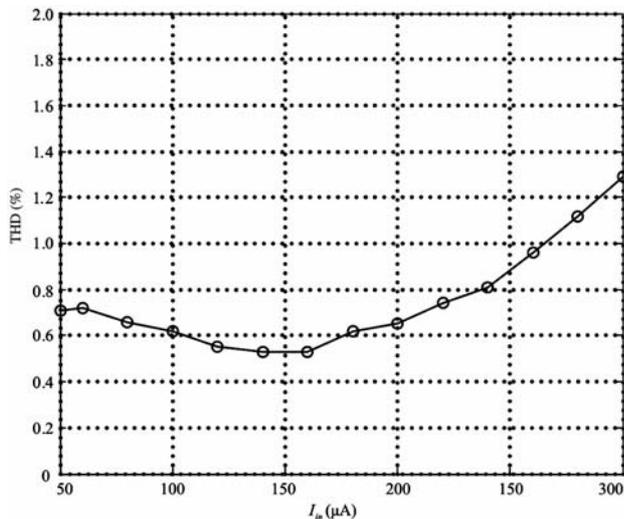
Fig. 12 — THD variation versus peak-to-peak amplitude of the applied sinusoidal input current
