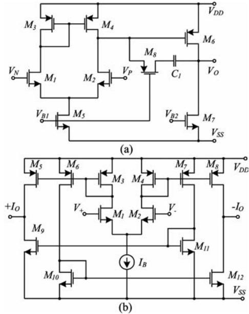
Fig. 4 — Schematic of CMOS (a) OA (b) OTA
