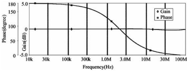
Fig. 7 — Gain and phase response of the proposed current-mode first-order APF
