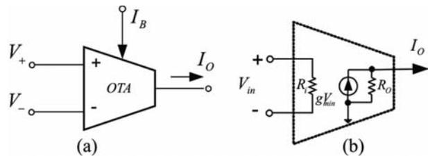
Fig. 1 — OTA (a) Symbol (b) Equivalent circuit
