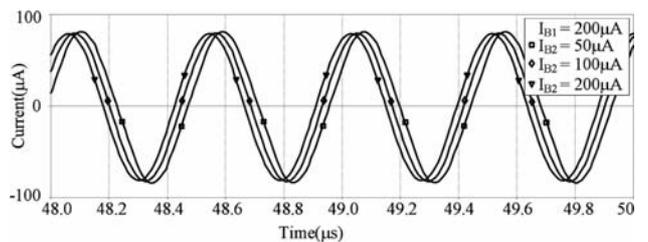
Fig. 11 — Output currents for difference values of  $I_{B2}$
