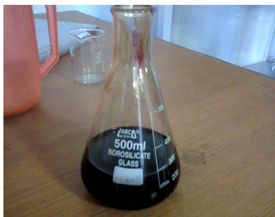
Fig. 9 — Graphene dispersion in ODCB (ortho dichloro benzene) solvent obtained by liquid phase exfoliation method
