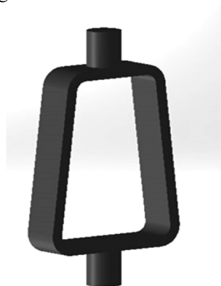
Fig. 1 — 3-D view of the force-sensing element of the transducer
