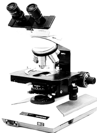
Fig. 3 – Photo of the Olympus BH-2 transmitted light-binocular microscope 4 .
