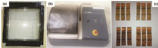
Fig. 3 — (a) Mould for specimen preparation (b) Specimen cutting machine (c) Fabricated Specimens
