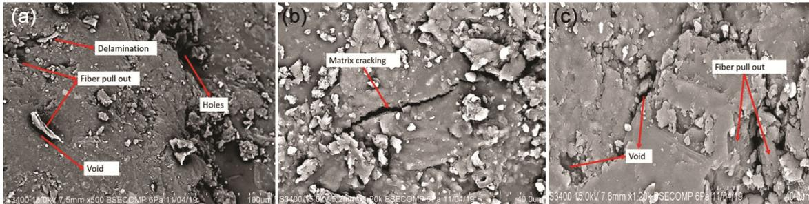
Fig. 6 — SEM images of the fractured sample surfaces
