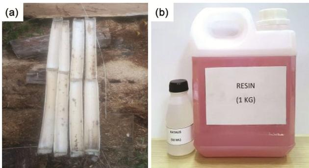
Fig. 1 — (a)Bambusa vulgaris (b) Unsaturated polyester resin and MEPK hardener
