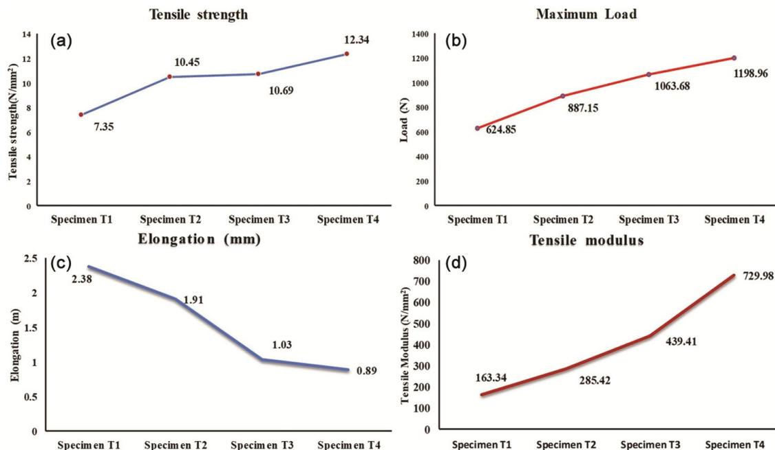
Fig. 5 — (a) Tensile strength (b) Maximum load (c) Elongation (d) Tensile modulus of the specimens
