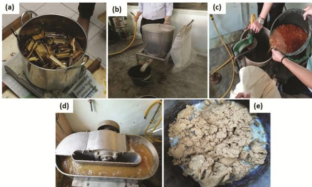
Fig. 2 — (a) Alkali retting (b) Hydro pulping (c) Screening (d) Beating (e) bamboo fibre
