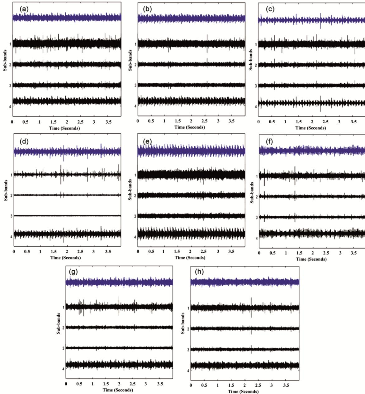
Fig. 3 — TQWT based decomposition of vibration signal of the gearbox (a) Label-1 (b) Label-2 (c) Label-3 (d) Label-4 (e) Label-5 (f) Label-6 (g) Label-7 (h) Label-8
