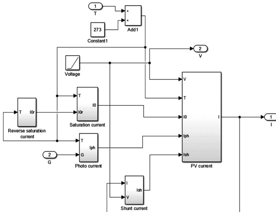
Fig. 4 — Simulation model of one diode
