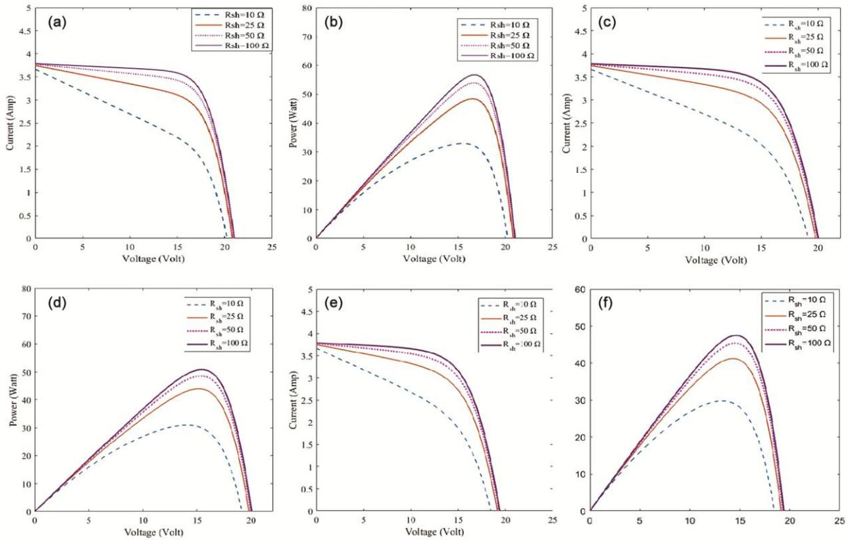
Fig. 11 — Effect of shunt resistance on I-V and P-V curve: one diode (a, b); double diode (c, d); triple diode (e, f)
