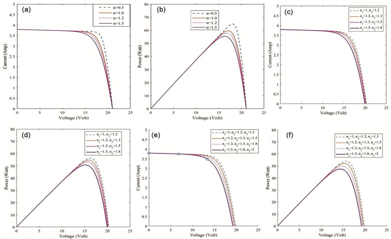
Fig. 9 — Effect of ideality factor on I-V and P-V curve: one diode (a, b); double diode (c, d); triple diode (e, f)
