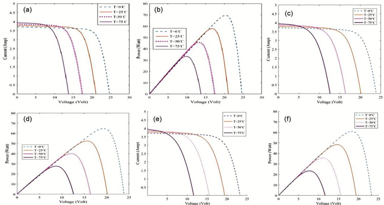
Fig. 7 — Effect of T on I-V and P-V curve: one diode (a, b); double diode (c, d); triple diode (e, f)
