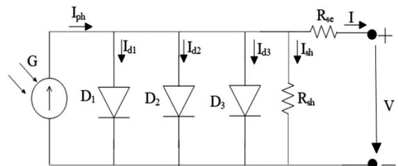
Fig. 3 — Three diode model
