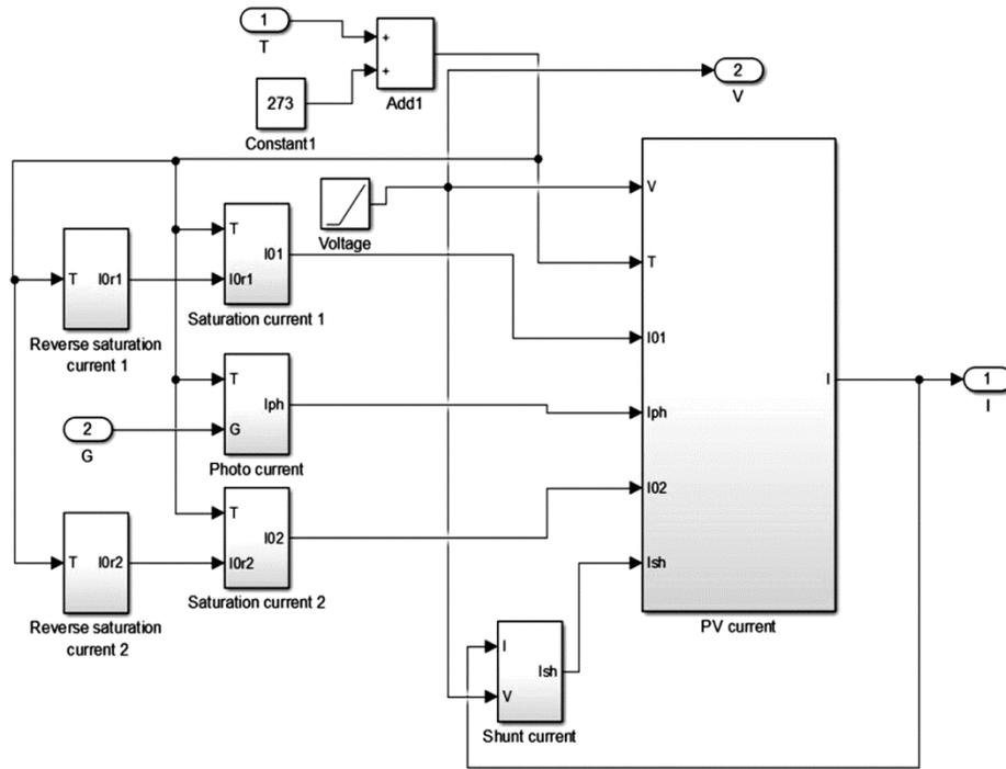
Fig. 5 — Simulation model of two diode model
