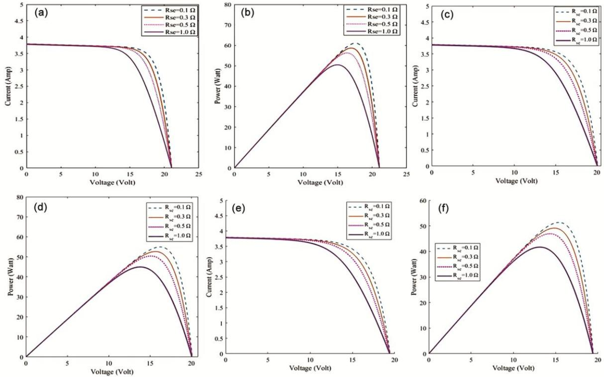
Fig. 10 — Effect of series resistance on I-V and P-V curve: one diode (a, b); double diode (c, d); triple diode (e, f)
