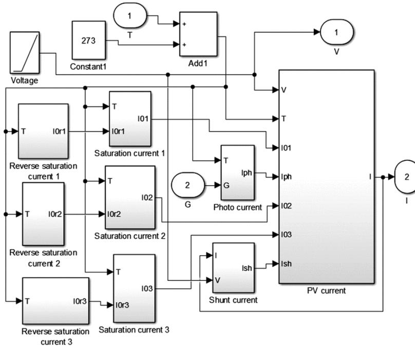
Fig. 6 — Simulation model of 3-diode model PV cell
