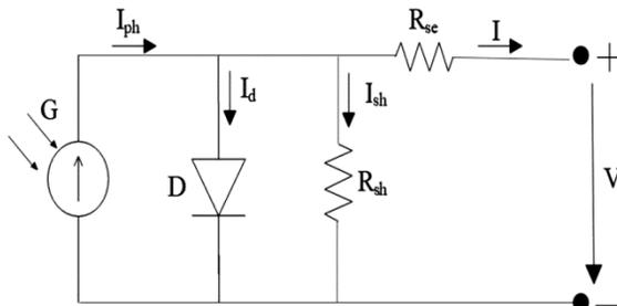
Fig. 1 — Practical form of one diode model
