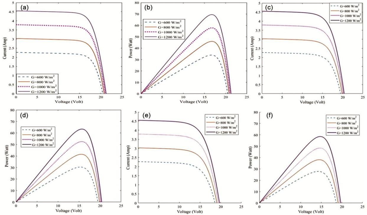
Fig. 8 — Effect of  $G$  on I-V and P-V curve: one diode (a, b); double diode (c, d); triple diode (e, f)
