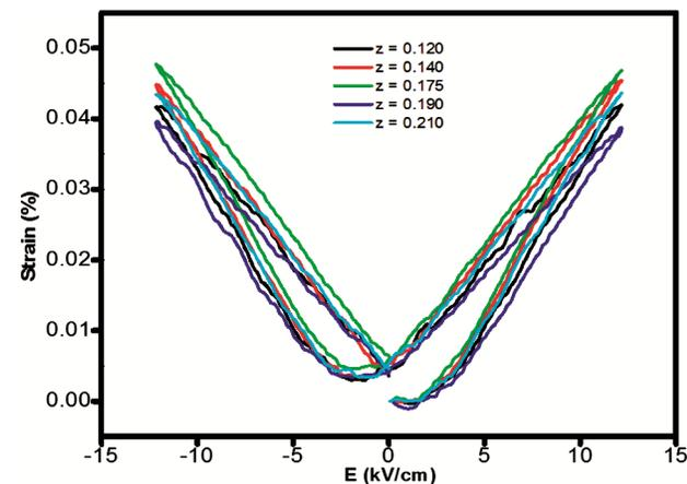
Fig. 9 — Plot of strain (%) with electric field, in  $\text{Na}_{1-z}\text{K}_z\text{NbO}_3$ , ( $0.120 \leq z \leq 0.210$ ) ceramics.
