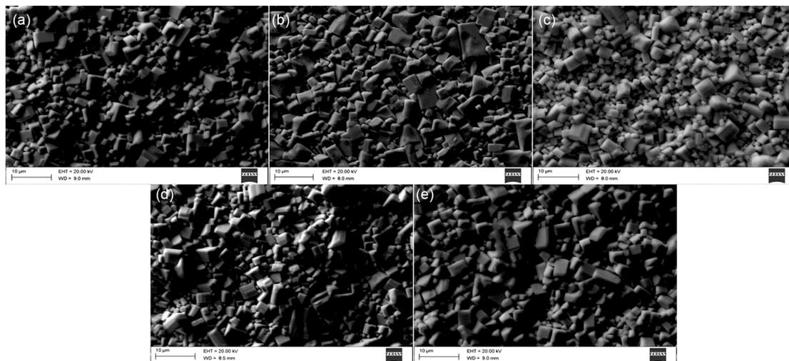
Fig. 4 — The SEM images of  $(\text{Na}_{1-z}\text{K}_z\text{NbO}_3)$  ( $0.120 \leq z \leq 0.210$ ) ceramics, (a)  $z = 0.120$ , (b)  $z = 0.140$ , (c)  $z = 0.175$ , (d)  $z = 0.190$ , (e)  $z = 0.210$ , respectively.
