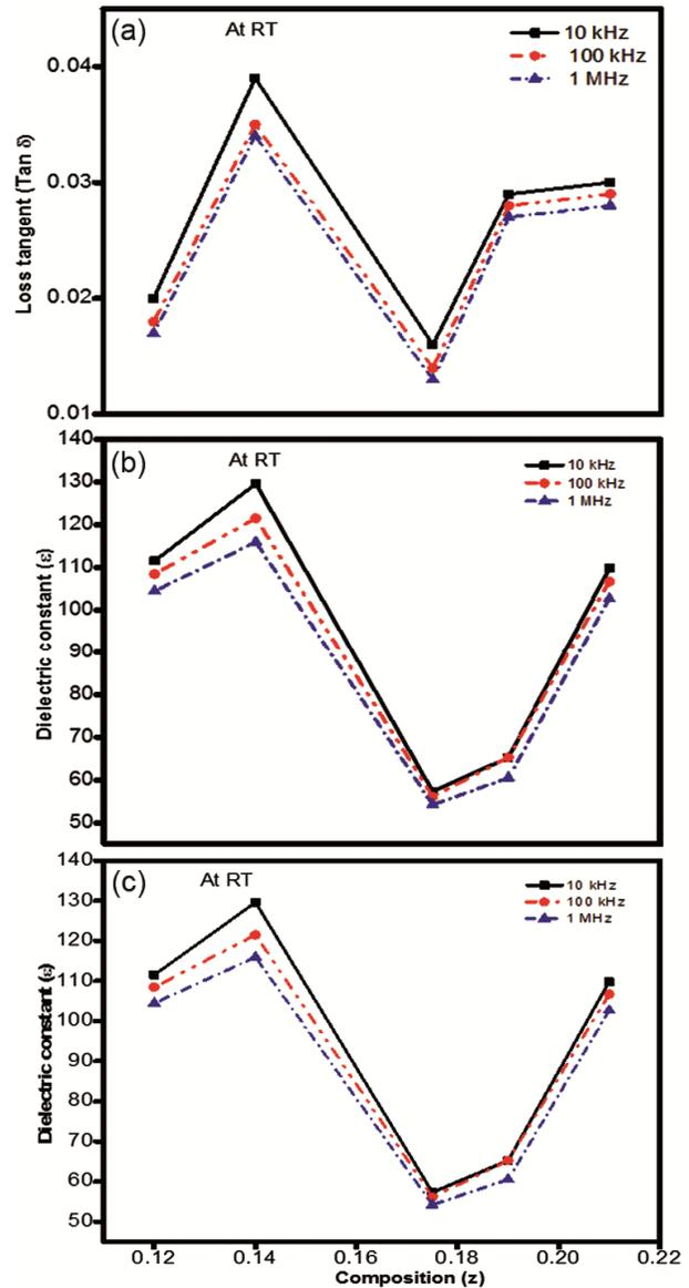
Fig. 7 — (a) Composition dependent loss tangent ( $\tan \delta$ ) of NKN ceramics, at different frequencies. (b) Composition dependent electric conductivity ( $\sigma$ ) of NKN ceramics, at different frequencies. (c) Composition dependent dielectric constant of NKN ceramics, at different frequencies.
