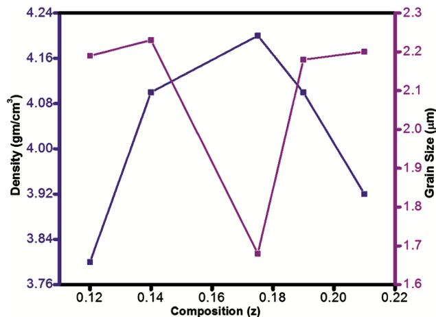
Fig. 5 — Variation of density and grain size with composition ( $z$ ), in  $\text{Na}_{1-z}\text{K}_z\text{NbO}_3$  ( $0.120 \leq z \leq 0.210$ ) ceramics.
