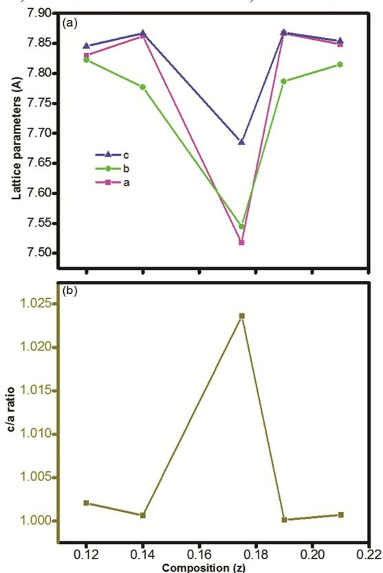
Fig. 3 — (a) Variation of Cell parameters with sample ( $z$ ), and (b) variation of  $c/a$  ratio with sample ( $z$ ), in  $\text{Na}_{1-z}\text{K}_z\text{NbO}_3$  ( $0.120 \leq z \leq 0.210$ ) ceramics.
