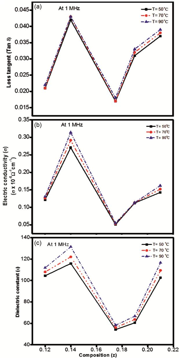
Fig. 6 — (a) Composition dependent loss tangent ( $\tan \delta$ ) of NKN ceramics, at different temperatures. (b) Composition dependent electric conductivity ( $\sigma$ ) of NKN ceramics, at different temperatures. (c) Composition dependent dielectric constant of NKN ceramics, at different temperatures.
