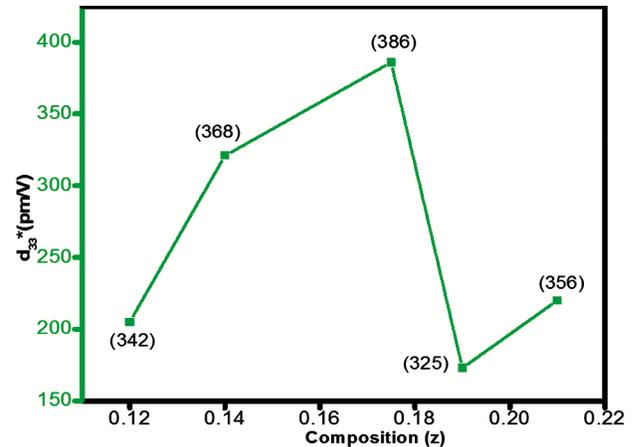
Fig. 10 — Plot of converse piezoelectric constant ( $d_{33}^*$ ) with sample ( $z$ ), in  $\text{Na}_{1-z}\text{K}_z\text{NbO}_3$ , ( $0.120 \leq z \leq 0.210$ ) ceramics.
