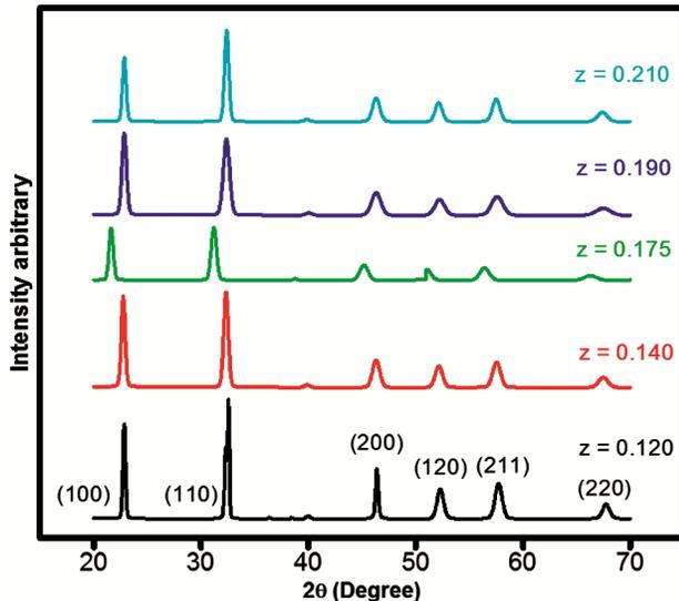
Fig. 1 — XRD patterns of the  $\text{Na}_{1-z}\text{K}_z\text{NbO}_3$  ( $0.120 \leq z \leq 0.210$ ) ceramics.
