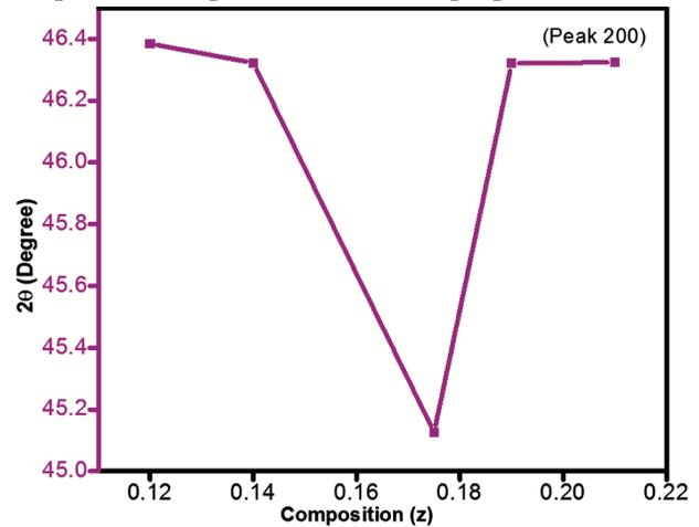
Fig. 2 — Peak (200) shifting tendency with sample ( $z$ ), in  $\text{Na}_{1-z}\text{K}_z\text{NbO}_3$  ( $0.120 \leq z \leq 0.210$ ) ceramics.
