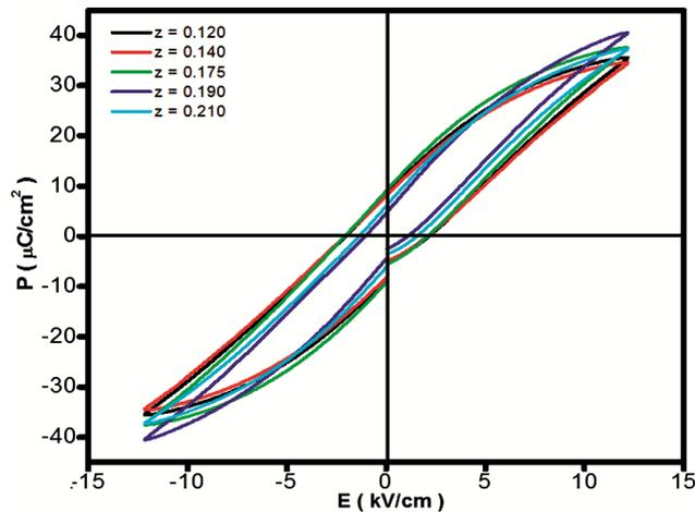
Fig. 8 — Polarization vs. electric field (P-E) hysteresis loops of  $\text{Na}_{1-z}\text{K}_z\text{NbO}_3$ , ( $0.120 \leq z \leq 0.210$ ) ceramics.
