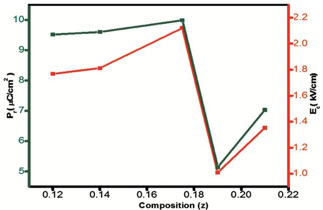
Fig. 11 — Variations of coercive field ( $E_c$ ) and remnant polarization ( $P_r$ ) with sample ( $z$ ), in  $\text{Na}_{1-z}\text{K}_z\text{NbO}_3$ , ( $0.120 \leq z \leq 0.210$ ) ceramics.
