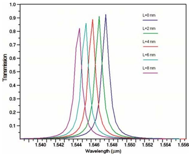
Fig. 7 — Output spectra of the filter for different values of  $L$ Table 2 — Significant parameters of the proposed filter for different values of  $N_d$
