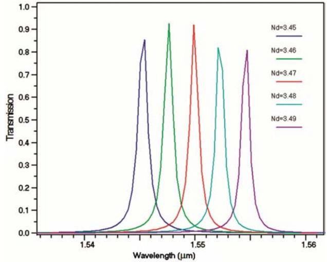
Fig. 6 — Output spectra of the filter for different values of  $N_d$
