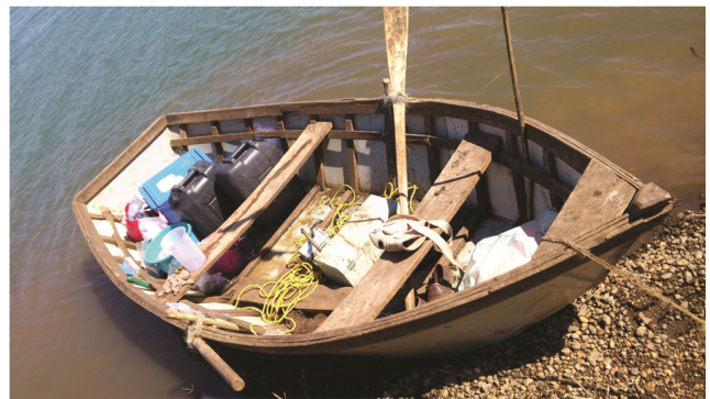
Fig. 5 — Plank built boat in water
