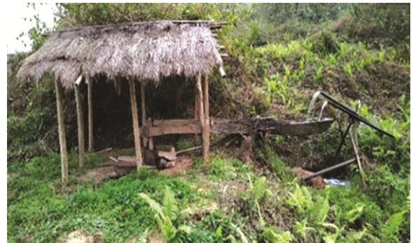
Fig. 9 — Water-operated husking lever ( tui-sum ) at its initial horizontal position where water started pouring in (Dahtum village, Henglep, Ccpur district, Manipur)
