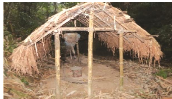
Fig. 12 — Resting the lever with an upright wooden pole and a mortar (15 kg oil tin) covered with a lid (Dahtum village)
