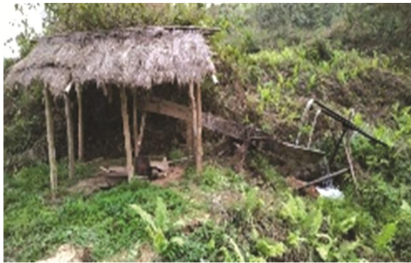
Fig. 10 — Semi-tilted position of the husking lever. Due to its tilted position small amount of water started pouring out of the water cavity
