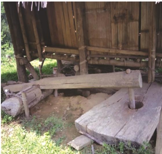
Fig. 7 — A leg-operated husking lever known as (chot-lep) (Khongmol village, Noney district, Manipur)
