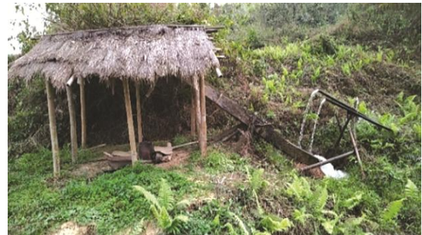
Fig. 11 — The husking lever tilted to its maximum torque and quickly emptied the water cavity
