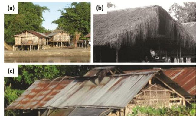
Fig. 10 — (a) Stilted structure built near river bank (b) thatch roof used in older houses (c) GI sheet sloping roof used currently
